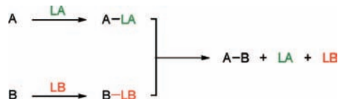
SCHEME 1. Bifunctional Lewis Acid/Base (LA/LB) Catalysis
